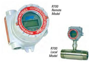
The R700 4-20 mA Transmitter is a loop powered transmitter with simultaneous Rate & Total indicator. The R700 features an explosion proof enclosure for hazardous location use. It also features 20 point linearization.
